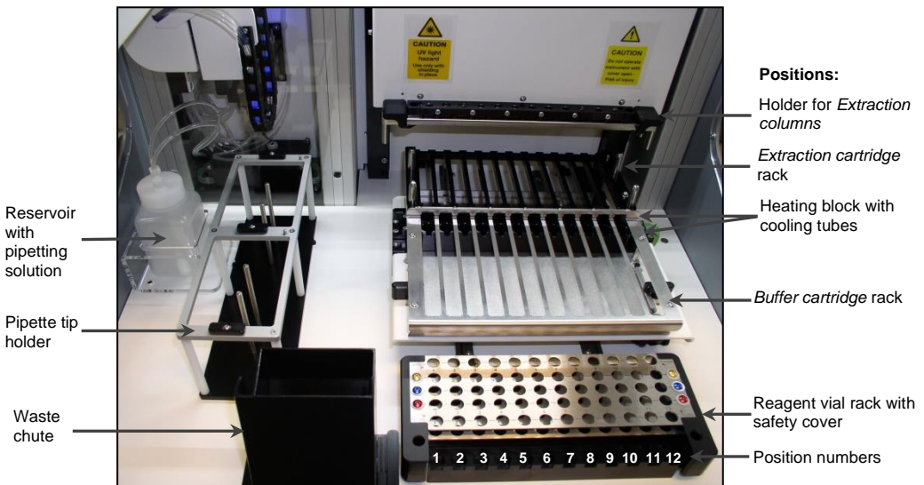
Fig. 3: The interior of the SelectNA™ plus instrument.
