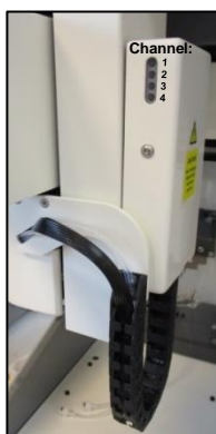
Fig. 4: Pipetting arm with new pressure monitoring system.
