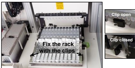
Fig. 21: Loading procedure of the filled buffer rack into the instrument.
