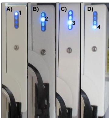
Fig. 5: Four channels of the pressure monitoring system. The blue LED is switched on if the corresponding sample position of the pipetting block is blocked.
