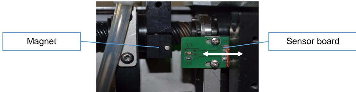
The sensor board can be slightly moved for the X-shift home position. For the proper board position the X arm stops after homing so that the aspiration tube is approximately in the centre of the priming bowl.
