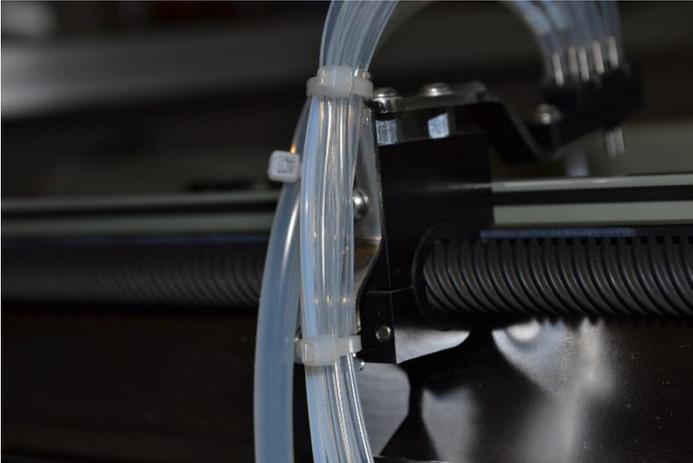
Put the binding spiral on the silikon tubes and move it to position according to the second picture.
