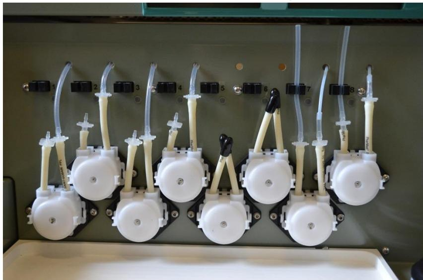
Put the tubes to the dispensing head according to the picture. Use the silikon tube conjunctions for the channels 7 and 8.
