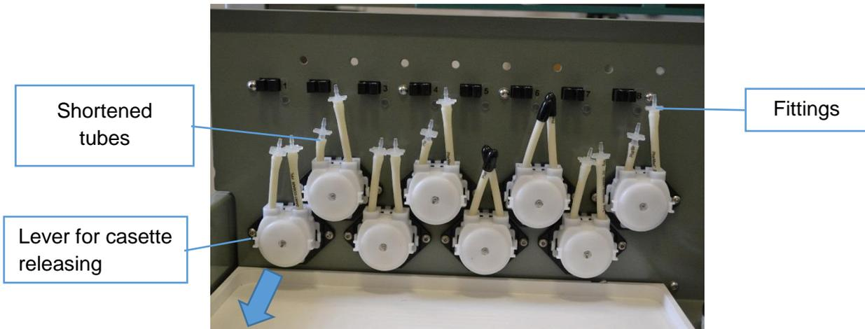
Put the silikon tube conjunctions to the pump 7 and 8 (it will be used for the teflon tube connection).
