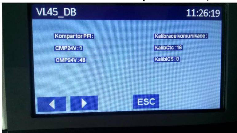
Komparator PFI – comparator of the power supply level used for the power supply failure handling
