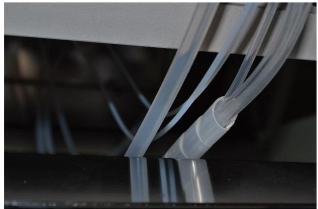
Put the bottle tubes with straws to pumps. Place it into the sensors bodies.
