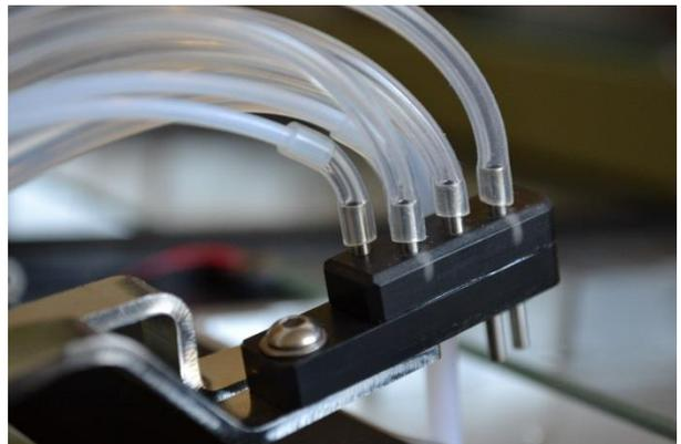
Secure the tubes to the holder on the back side of the x-shift arm. Use the plastic bindings.
