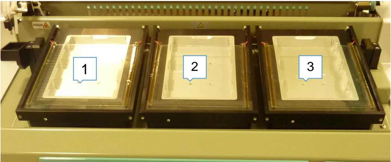
When you look for the block current address disconnect the power connectors of the other two blocks. (Note : The new spare heated block are set to address 1).
