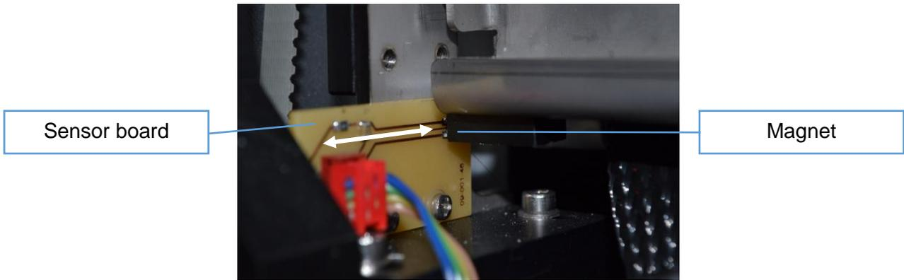
The sensor board can be slightly moved for the aspiration arm home position. For the proper board position the aspirating tube stops in upper position so it does not hit other parts during X-shift movement.
