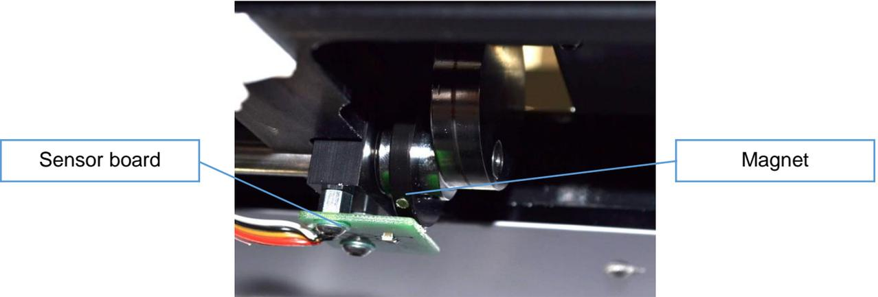
The magnet is placed in the plastic wheel. It is secured on the eccentric pivot with a small screw. For the proper plastic wheel position the tray holder stops very near to the horizontal position which comes after the holder passes upper position (the eccentric turns counterclockwise).
