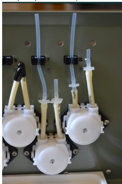
Put the silicon and teflon tubes to all pumps and push it through the holes into the instrument inside.
