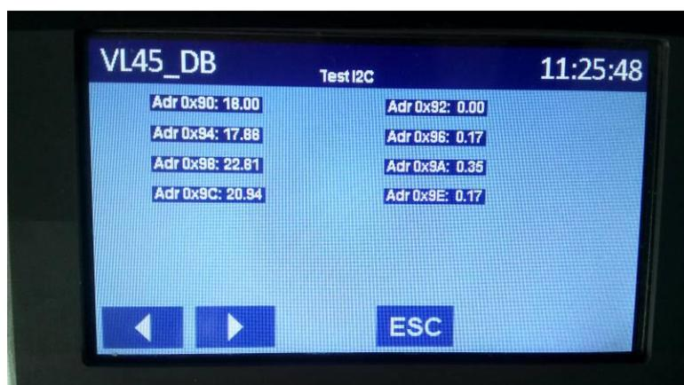
The temperature values at the address lines are assigned to sensors related to setting of the menu Setup / 02 Reag positions sensors :
